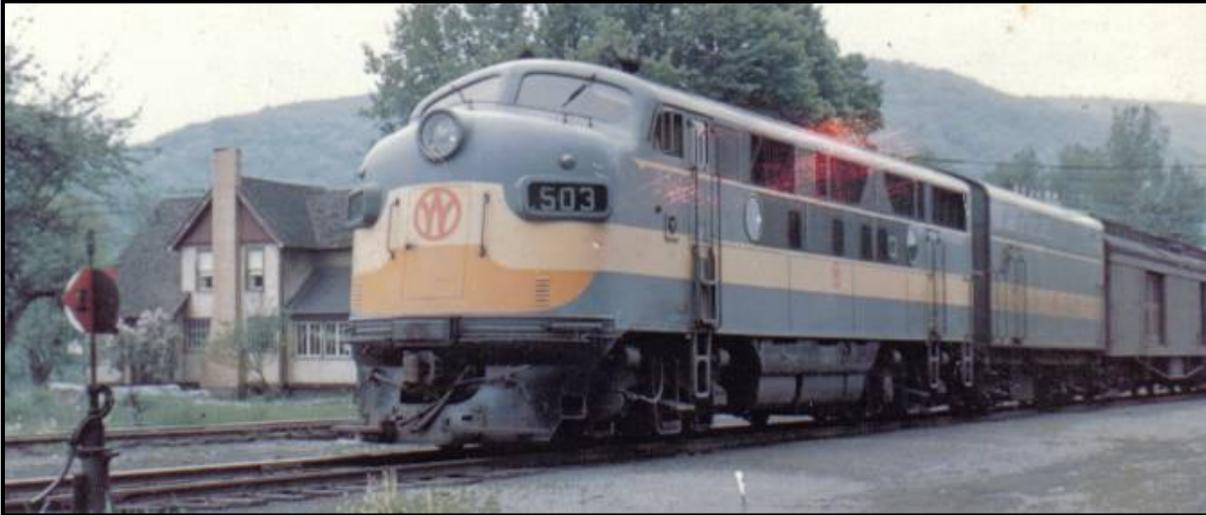
F-3 #503 with Train #2 nears Roscoe with Heater CAR HT-2 in the consist. The O&W, like many other railroads, used heater cars to provide steam to keep passengers warm while maintaining maximum power control flexibility through the waning years of passenger service.
