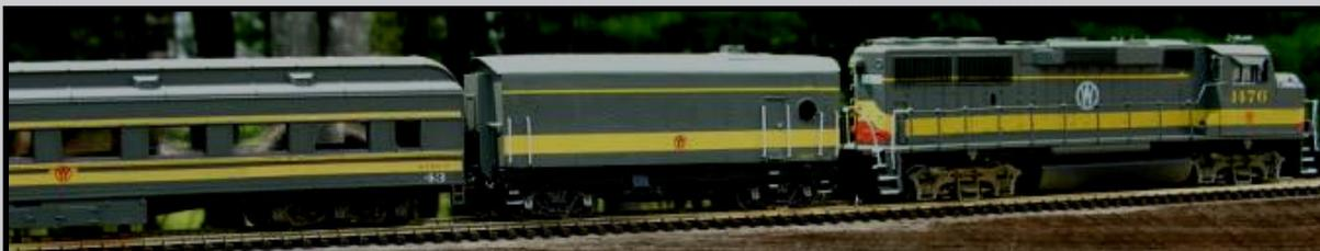
The finished model "Dullcoted" but before weathering. I followed modern practices that use safety white for railings, grabs, and step surfaces.
